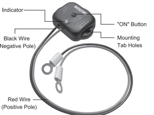
3. For vehicles - With the included cable ties, mount the Monitor to battery cable, and make sure that the mounting location is close enough to attach the two wires to the battery +/- terminals. For other devices, determine the best mounting location that doesn't interfere with the product in use.
